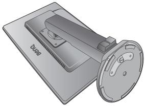
Extend the monitor to the maximum extended position. Then tilt the monitor. And rotate the monitor 90 degrees counterclockwise as illustrated.
